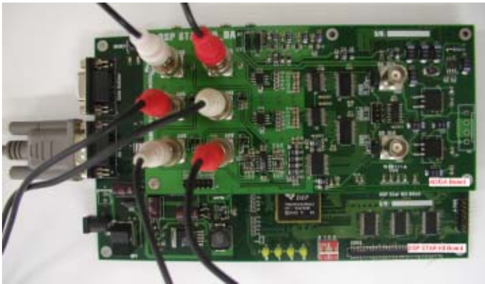
Figure 1. Installation of AD/DA with DSP STAR Kit board
