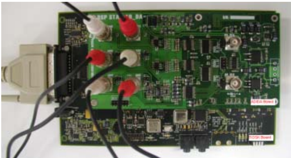
Figure 2. Installation of AD/DA with TI DSK board
